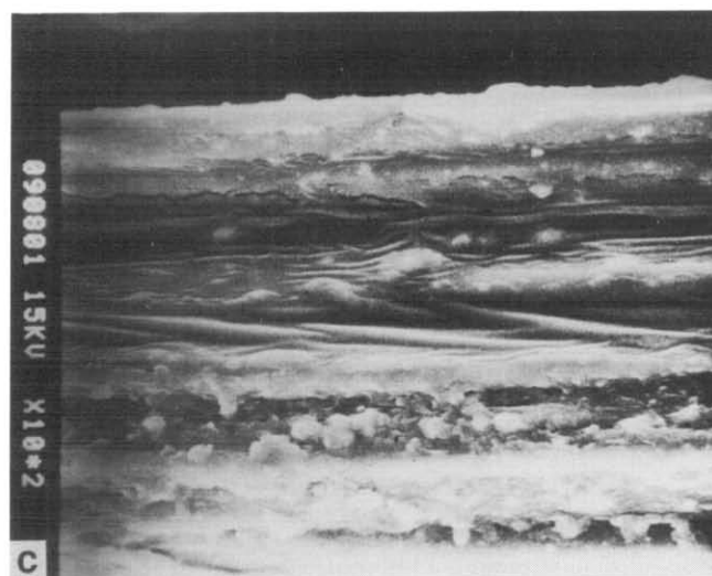
Figure 7 SEM micrographs showing surface morphology of different fibre samples: (a) \text{NaIO}_4 -treated DJ; (b) 15% PMMA-grafted DJ; (c) 30% PMMA-grafted DJ
